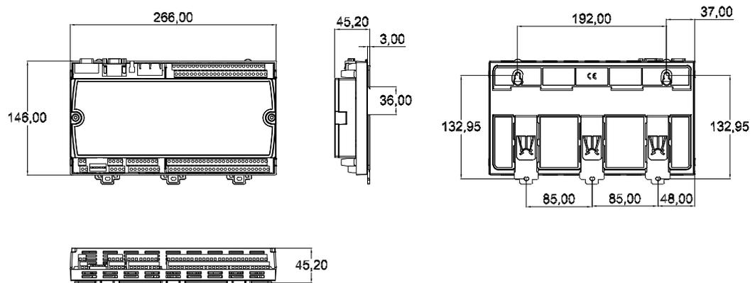
Figure 1.1 ECU-1911 Chassis Dimensions
