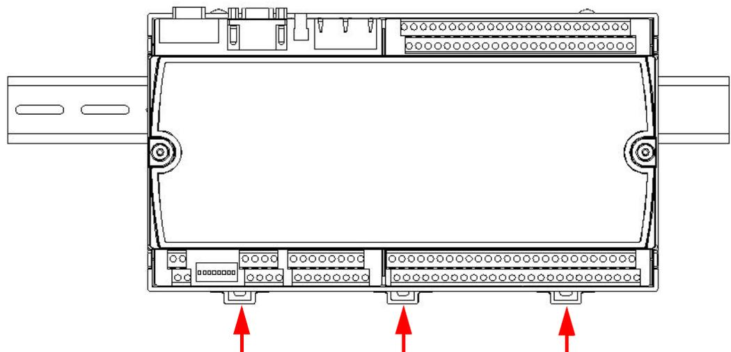
**Figure 3.2 Small bracket installation location**
