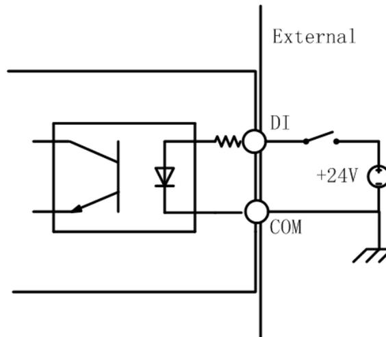
**Figure 2.8 Digital input connection (wet contact)**
