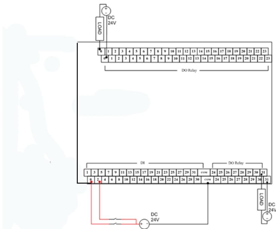
Figure 2.7 Digital input/output pin assignments
