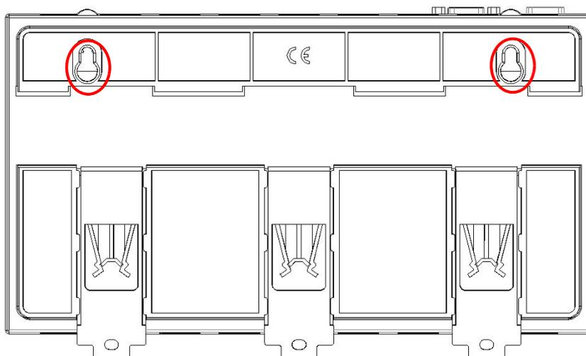
**Figure 3.4 ECU-1911 Wall-mount installation location**
