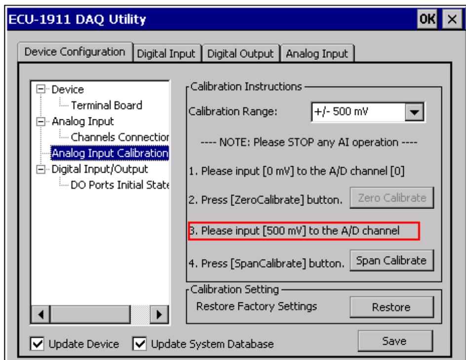
**Note!** *It is important that the accuracy after calibration depends on the DC source's accuracy.*
