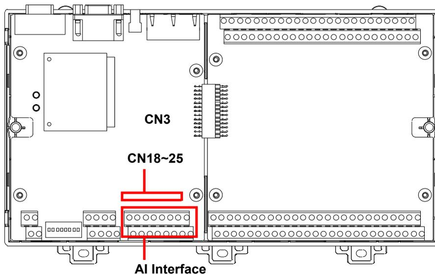
**Figure 2.11 Locations of Jumpers (CN18~25) and AI interface**
