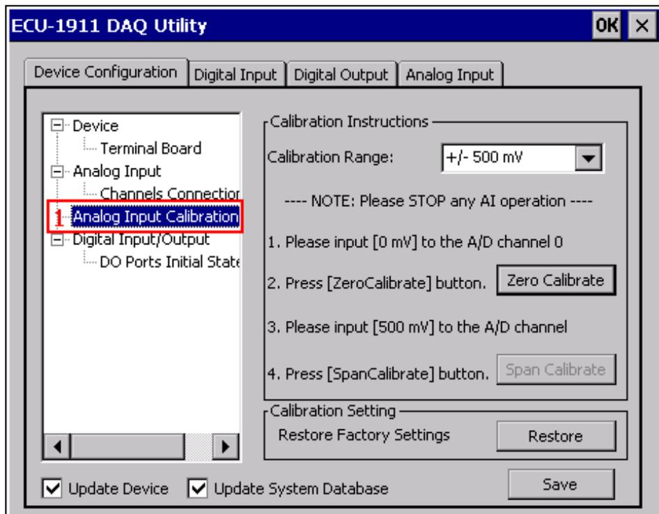
**Item1:** Display Analog Input Calibration (A/D Calibration).
