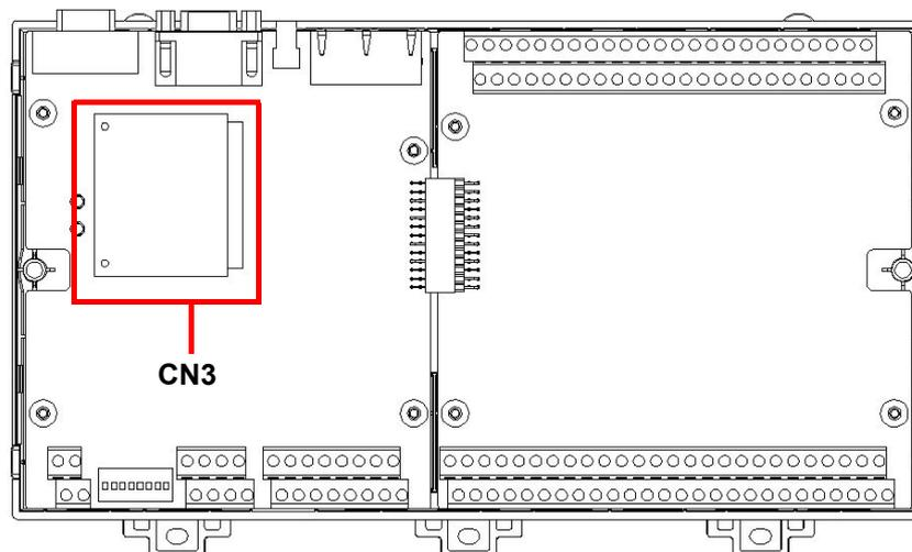
Figure 3.9 CompactFlash card slot location (CN3)
