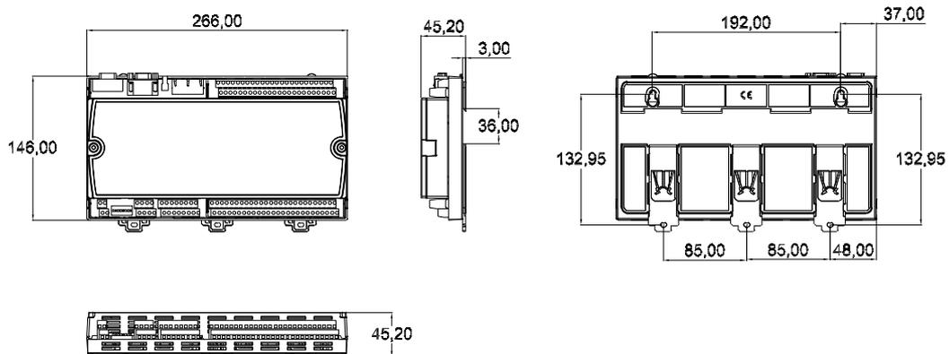
**Figure 3.3 ECU-1911 Wall-mount installation size**
