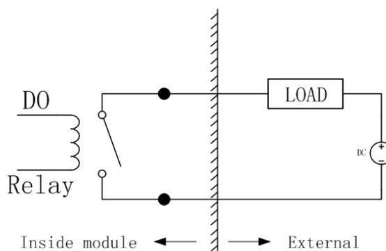
**Figure 2.9 Digital output connections (relay contact)**
