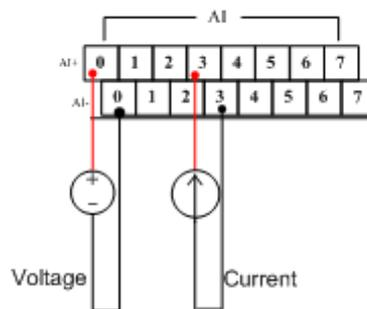
**Figure 2.10 Analog input pin assignments**
