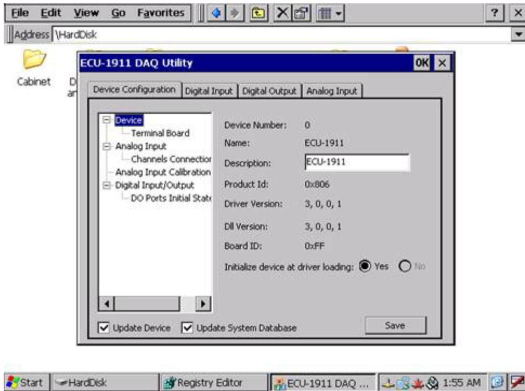
On the device setting dialog box, you can change default settings of Device, Analog Input, Digital Input/Output functions.
