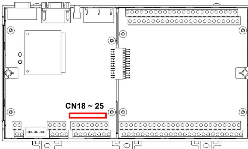
Figure 3.7 Jumper location (CN18 ~ 25)
