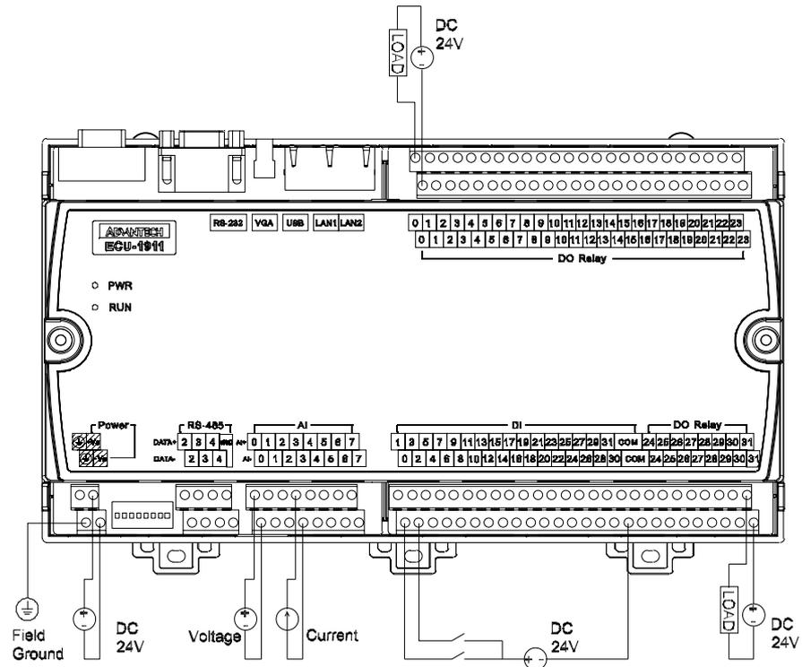
**Figure 3.11 ECU-1911 Field wiring signal**
