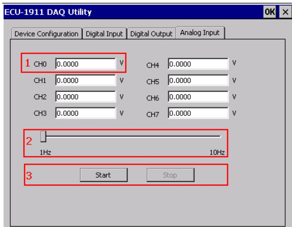
**Item 1:** Shows the sample data of a corresponding analog input channel. The user can select the value range type in the "Device Configuration" tab.
