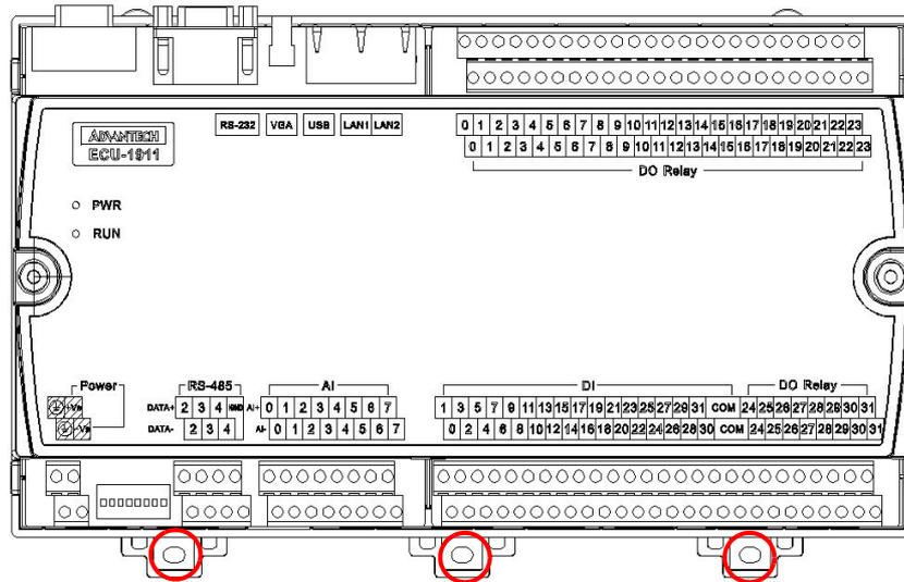
**Figure 3.5 ECU-1911 Wall-mount fix installation location**
