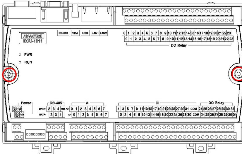
Figure 3.6 ECU-1911 top view location
